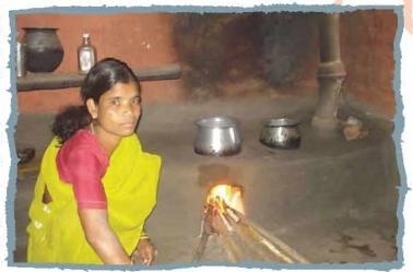
hazards, to be less dependent on firewood and to spend less time on collection of firewood as this model consumes less and less wood for cooking and erupting very low smoke which passes through a pipe over the roof of the house.
